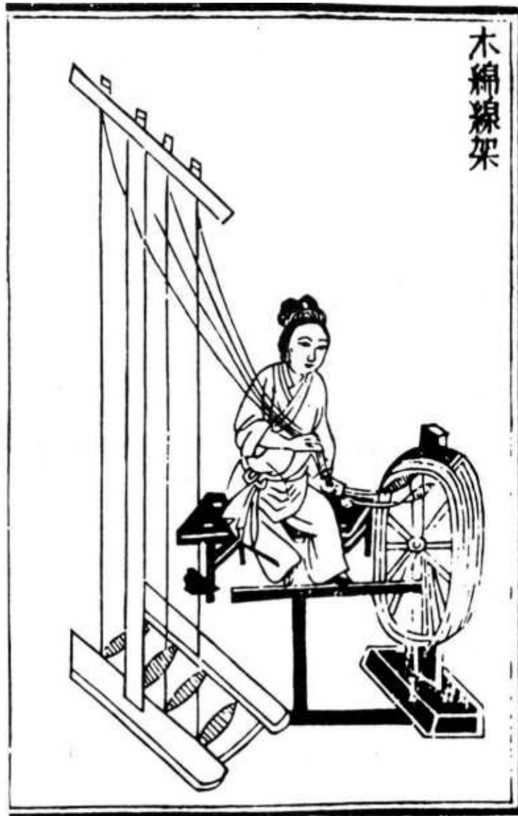
Figure 44. Spindle wheel for doubling (twisting together two separate yarns). The wheel is operated by it treadle.
